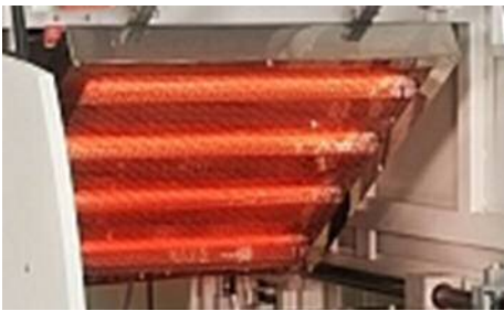
TOP SIDE PREHEAT UNIT
